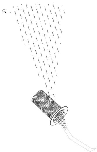
13. Despite cleaning with brush, if the stubborn dirt is not washed off, then the filter element must be cleaned with high pressure water wash
