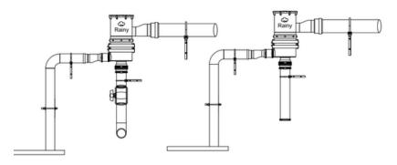
1. ·Avoid installing a ball valve or an end cap at the drain water outlet since this filter has an open-ended design
