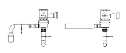
5. Avoid undue increasing the diameter of the pipe using additional reducers and increasers
