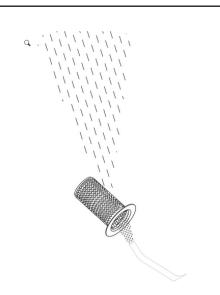
13. Despite cleaning with brush, if the stubborn dirt is not washed off, then the filter element must be cleaned with high pressure water wash
