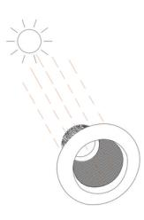
12. After cleaning, lift the filter element and observe under sunlight, light should pass through the filter element sieve. If light passes, re insert the filter element.
