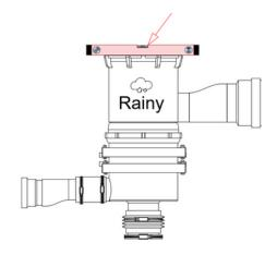
3. Confirm that the filter is securely affixed and aligned using a spirit level.
