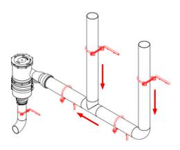
4. The pipe connecting to the filter's inlet should have a downward slope.
