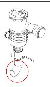
9. Install an elbow at the drain water outlet.
