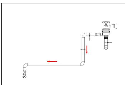
5. Maintaining the appropriate gradient for the clean water outlet is necessary.
