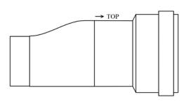
14. While installing the eccentric reducer ensure the top sign is facing upwards.
