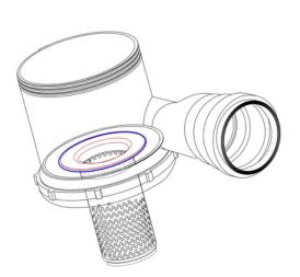
11. The SS 304 screen must be correctly and firmly installed within the allocated groove in the upper housing of the filter, ensuring that no gaps exist between the screen and the provided groove.
