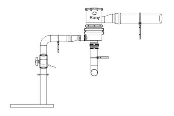
8. If you opt to install ball valve at the clean water outlet, position it on the vertical pipe.
