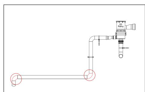
7. If the clean water outlet has an extended length, connect it using two elbows while maintaining the necessary gradient.
