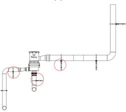
2. Ensure the attachment of an 'L' clamp at the inlet pipe, clean water outlet, and drain water outlet
