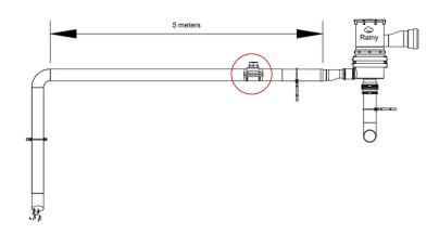
6. In case the clean water inlet is longer than 5 meters, provide an air-vent on the pipe to maintain free gravity flow .
