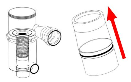
10. The intermediate bush, should be securely positioned with its narrower end facing upward, affixed to the bottom of the screen, and its broader side oriented downward, firmly secured to the lower body of the filter.
